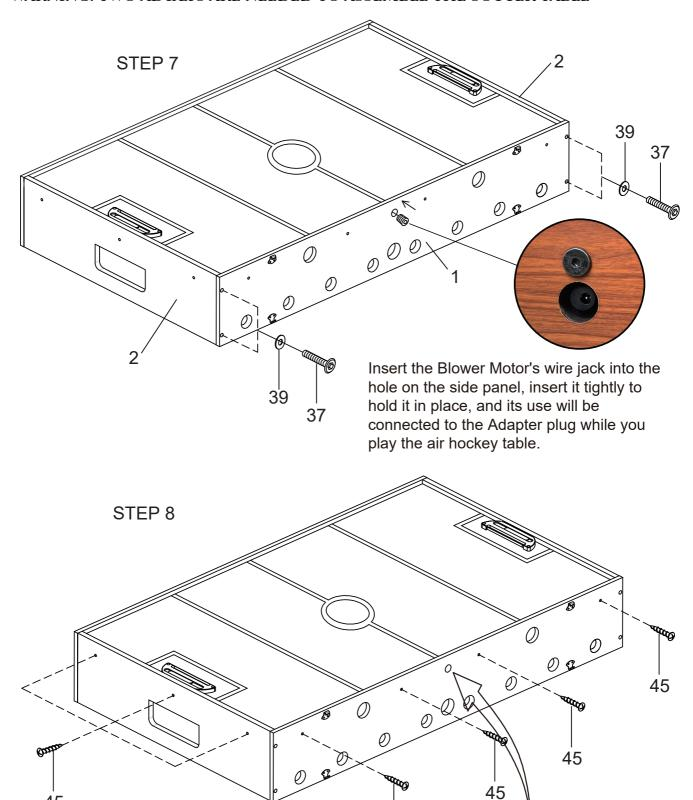
The Blower Motor jack into the hole on the side panel, which will be used to connect to the Adapter (#34).
