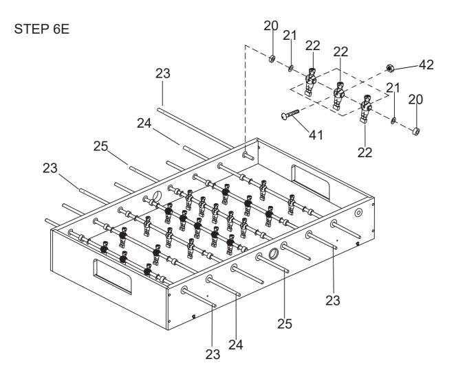
Insert the rod end part way through one side panel, and then place the rest of the parts needed on each rod, in the order shown, before inserting through the other side panel.
