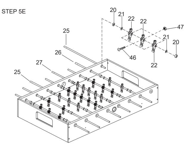
Insert the rod end part way through one side panel, and then place the rest of the parts needed on each rod, in the order shown, before inserting through the other side panel.
