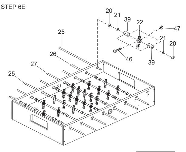
Insert the rod end part way through one side panel, and then place the rest of the parts needed on each rod, in the order shown, before inserting through the other side panel.
