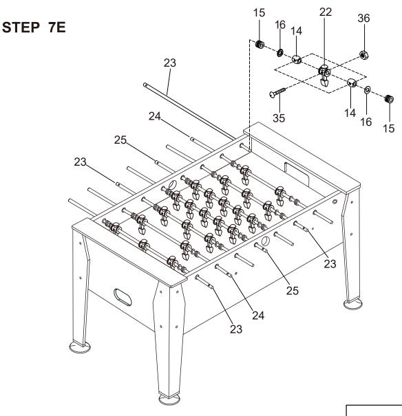
Insert the rod end part way through one side panel, and then place the rest of the parts needed on each rod, in the order shown, before inserting through the other side panel.
