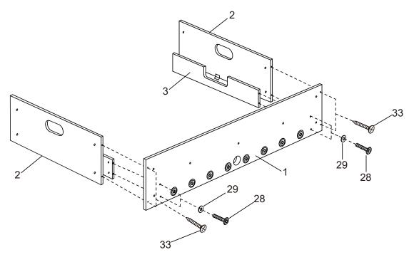
Attach the other one of the 2 Side Panels (#1) to the End Panel (#2) and Goal Board (#3) by using the Screw (#33), Bolt (#28), and the Washer (#29).
