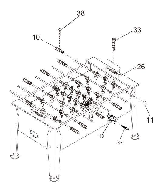
NOTE: Handle (10) attaches to rod end with hole and Rod End Cap (11) goes on opposite end. Each team should face the opposite goal and all be the same color.
