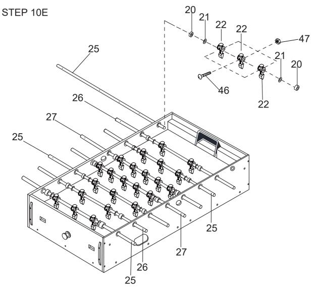
Insert the rod end part way through one side panel, and then place the rest of the parts needed on each rod, in the order shown, before inserting through the other side panel.
