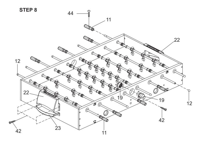
NOTE: Handle (11) attaches to rod end with hole and Rod End Cap (12) goes on opposite end. Each team should face the opposite goal and all be the same color.
