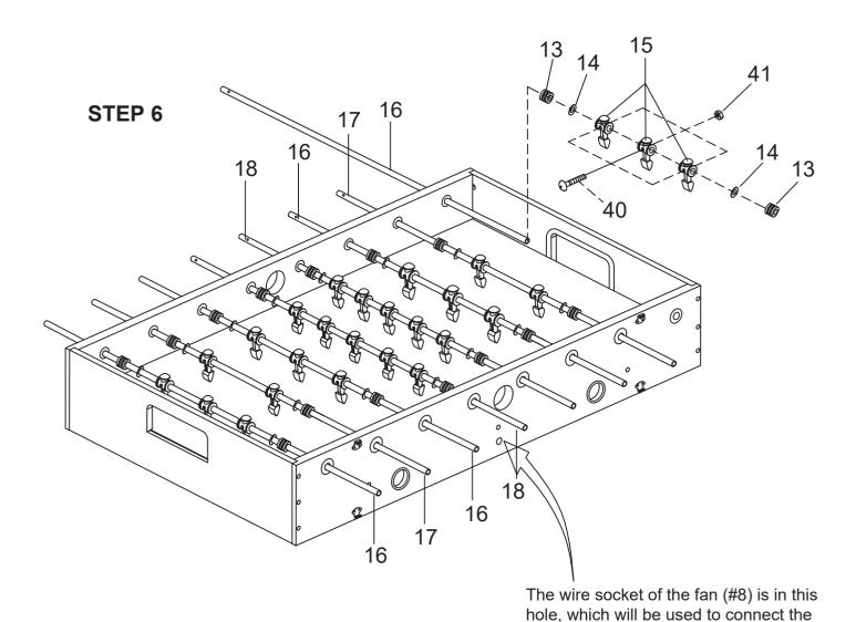
Insert rod end part way through one side panel, then place rest of parts needed on each rod, in order shown, before inserting through other side panel.
