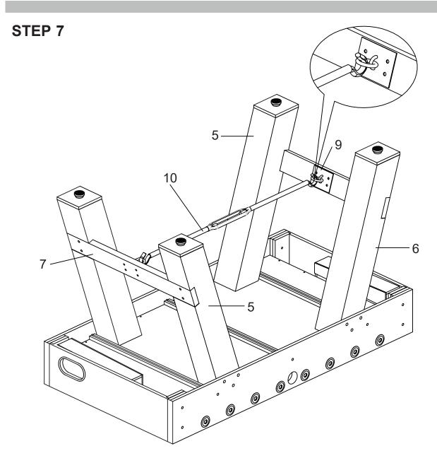
NOTE: Attach two ends of the Adjustable Support Bar (10) to the Ring Plates (9) on the Leg Panels. Adjust the length as necessary to fit.
